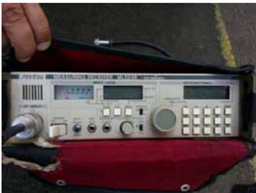
Gambar 3. Alat Ukur Field Strength
